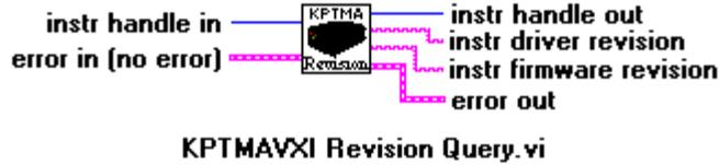
The RevisionQuery function returns the firmware revision of the Kepco TMA VXI-27 power supply controller and the revision of the Kepco Instrument driver.
