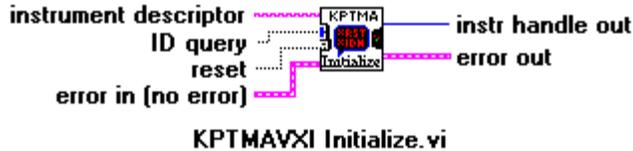
The Initialize function may be used when AutoCon is not needed. It is a low level function which requires an Instrument Descriptor, which includes the logical address of the Kepco controller. It is recommended that [AutoCon](#) be used instead.
