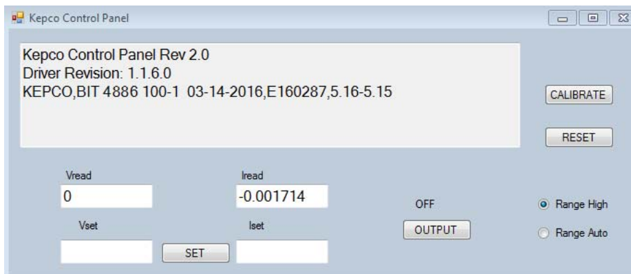
FIGURE 3-4. MAIN CONTROL PANEL, TYPICAL FOR BOP 100-1M WITH BIT 4886
