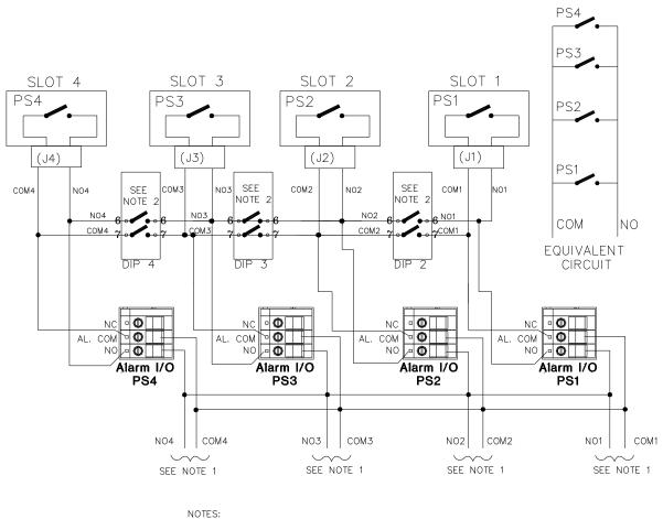
1. USE ANY PAIR OF NO() AND COM() LINES FOR CLOSE ON FAILURE ALARM. SET ALL ASSOCIATED DP SWITCHES, POSITIONS 6 AND 7, TO ON (CLOSED).
