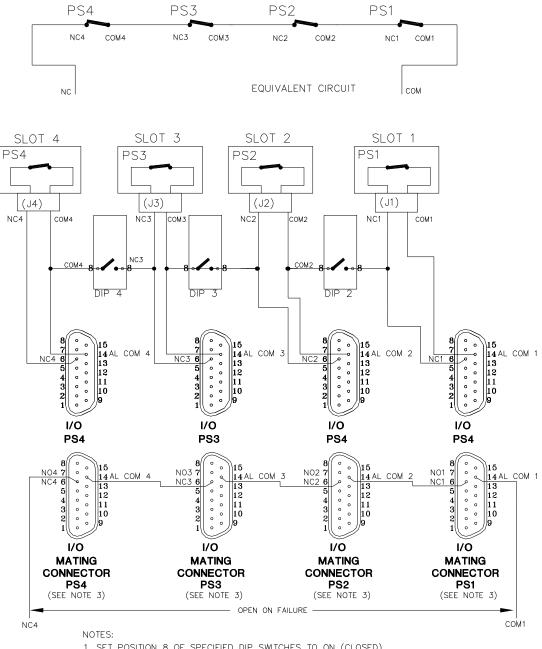
1. SET POSITION 8 OF SPECIFIED DIP SWITCHES TO ON (CLOSED).
