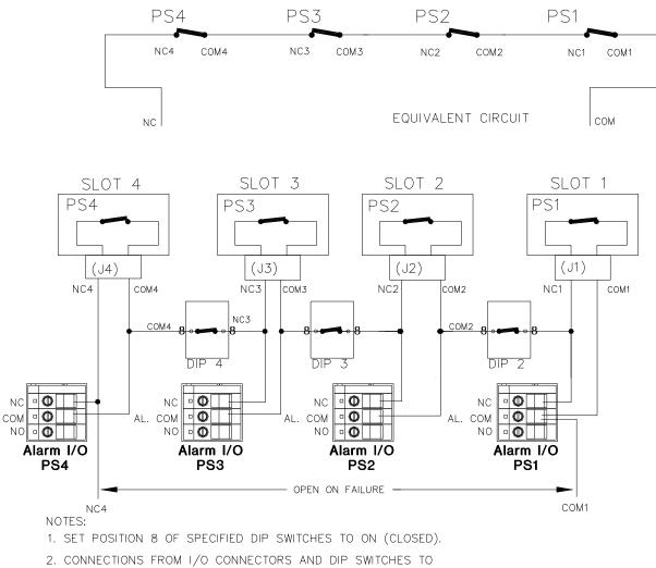
ALARM I/O TERMINAL BLOCKS ARE INTERNAL AND SHOWN FOR REFERENCE ONLY.
