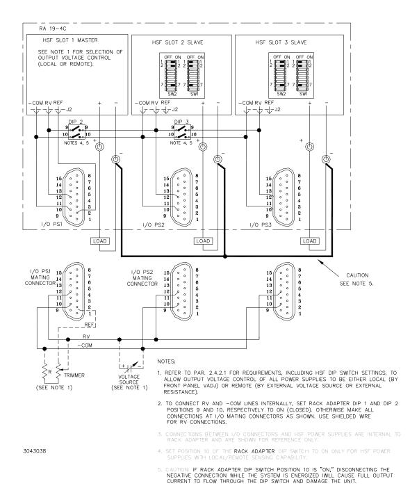
FIGURE 2-2. CONTROLLING MULTIPLE POWER SUPPLIES, MULTIPLE LOADS
