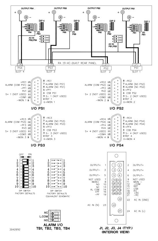
FIGURE 1-3. RA 19-4C-26417 REAR PANEL INTERCONNECTIONS
