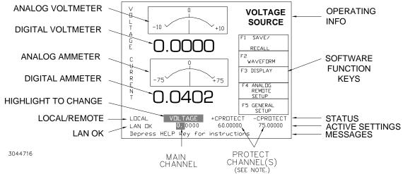
NOTE: WHEN SET TO BIPOLAR, ONLY ONE PROTECTION FIELD IS DISPLAYED. WHEN SET TO INDEPENDENT, TWO PROTECTION FIELDS ARE DISPLAYED AS SHOWN HERE. SEE PAR. 3.3.3.1 FOR DETAILS.
