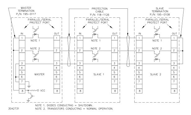
FIGURE 2-16. TYPICAL MASTER/SLAVE PROTECTION INTERCONNECTIONS
