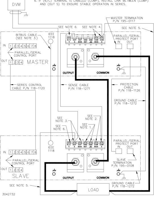
FIGURE 2-15. SERIES CONFIGURATION, REMOTE SENSING, TYPICAL
