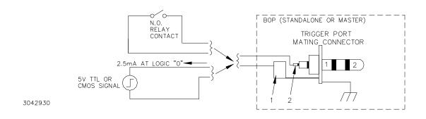
FIGURE 3-19. REMOTE STANDBY, STANDALONE OR MULTIPLE UNITS
