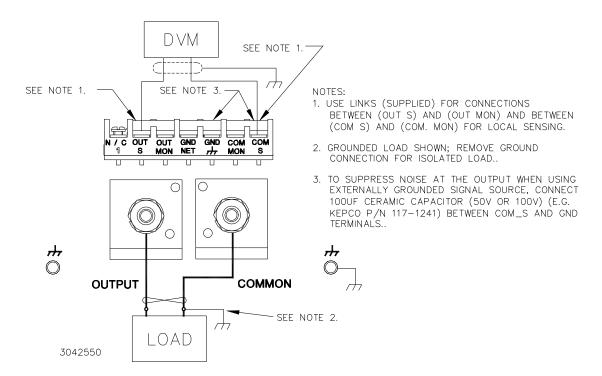
FIGURE 2-4. LOAD CONNECTIONS, LOCAL SENSING
