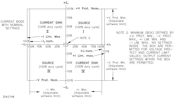
NOTE 3. The concept of "box value" is illustrated above. It is an area around the origin, where the limits of the unit (voltage or current) cannot be programmed. This minimum (box) value for the positive limits or maximum (box) value for the negative limits, is a model dependent constant of approximately 0.2% of the nominal values for voltage and current. The parameters involved are defined by Note 1 for voltage and Note 2 for current mode, and are further explained in Tables 3-4 and 3-5.
