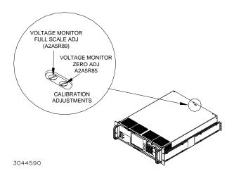
FIGURE 2-2. BOP1KW-MEL/MGL TOP COVER ACCESSIBLE COMPONENTS
