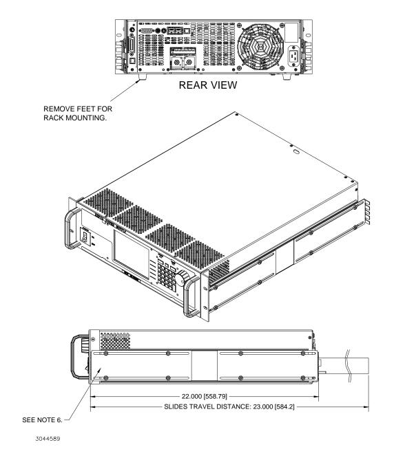
FIGURE 1-2. BOP POWER SUPPLY, OUTLINE DRAWING (SHEET 2 OF 2)
