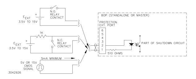
FIGURE 3-15. REMOTE SHUTDOWN USING EXTERNAL POWER, FOR STANDALONE OR MULTIPLE UNITS
