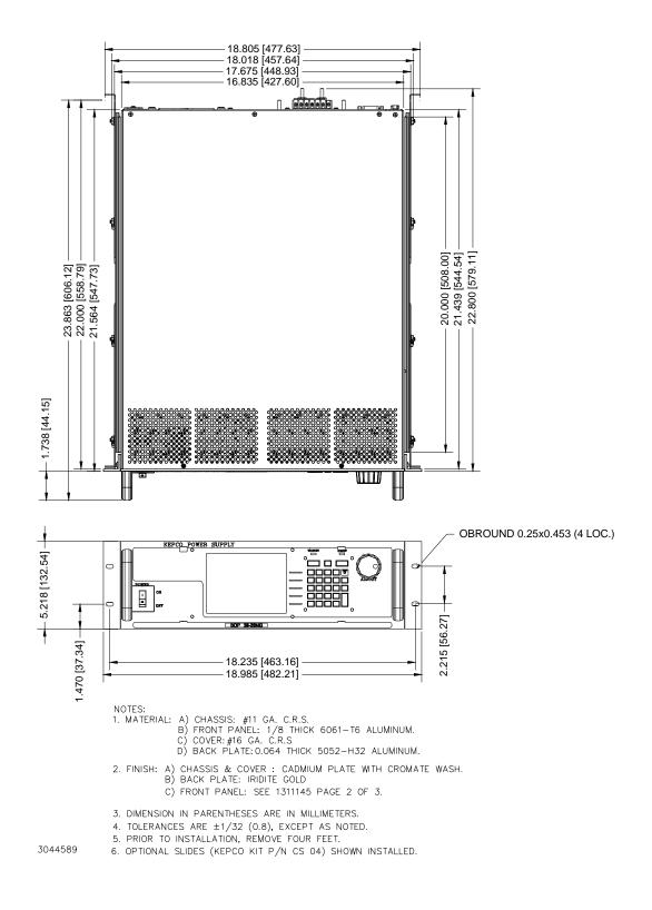
FIGURE 1-2. 1000W BOP POWER SUPPLY, OUTLINE DRAWING (SHEET 1 OF 2)
