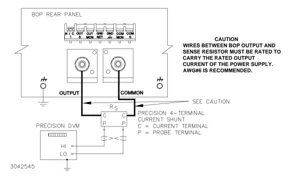
FIGURE 4-2. CALIBRATION SETUP FOR CURRENT MODE
