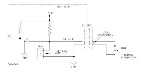
FIGURE 2-6. FAIL SAFE FEATURE, SIMPLIFIED SCHEMATIC DIAGRAM
