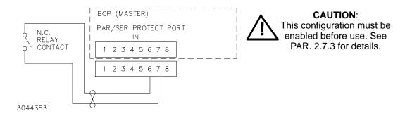
FIGURE 3-17. REMOTE SHUTDOWN COMBINED WITH CABLE-DISCONNECT SHUTDOWN, FOR STANDALONE OR MULTIPLE UNITS,
