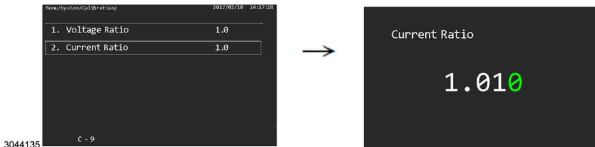
FIGURE 4-4. CURRENT RATIO CALIBRATION
