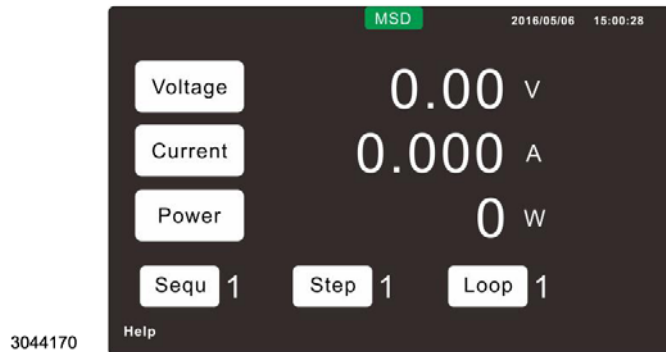
FIGURE 3-14. HOME SCREEN AFTER UPLOADING SEQUENCE FILE(‡)
