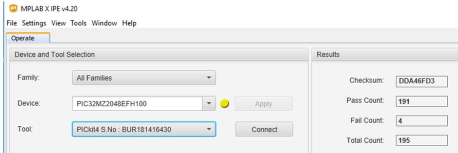
5. Click **Apply**, then click **Connect**. The firmware for the processors will be downloaded to the PICKit Programmer and then the Programmer will connect to the chip on the board. The output window shows the status (see Figure 5). Note that DSVSN information is unique to each chip.
