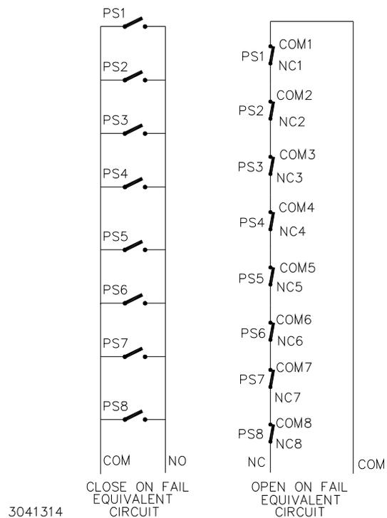
**FIGURE 3. TYPICAL ALARM CIRCUIT DIAGRAMS**
