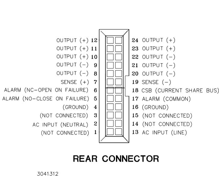
**FIGURE 2. REAR CONNECTOR PIN ASSIGNMENTS**
