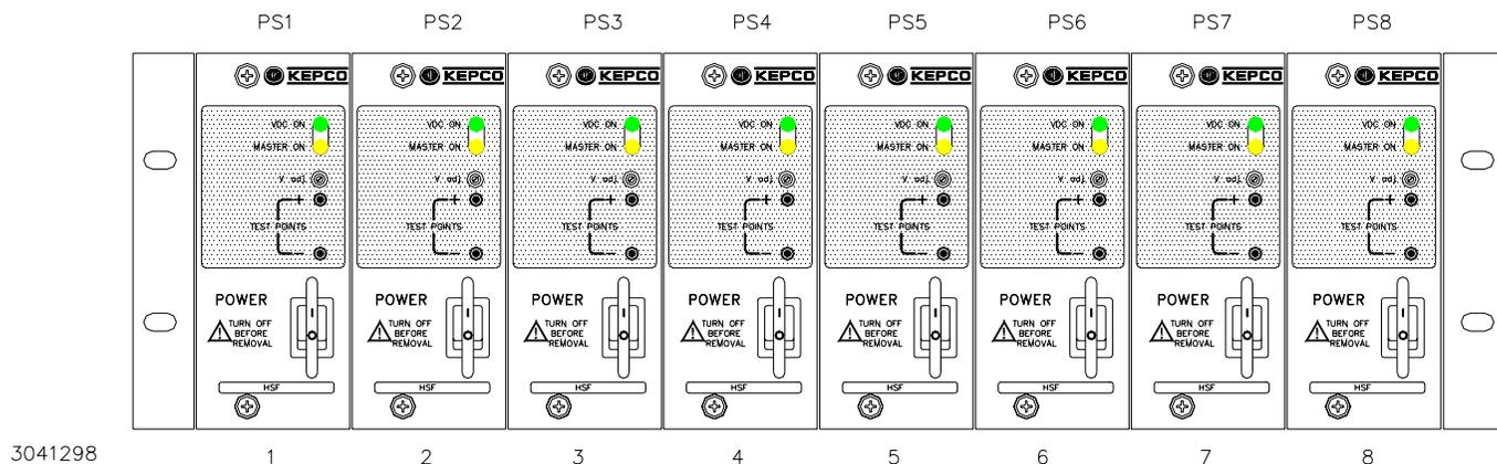
**FIGURE 1. HSF 50 WATT POWER SUPPLIES (8) INSTALLED IN RA 19-8B RACK ADAPTER**
