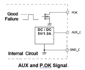
Open drain signal low when PSU turns on, Max. P.OK sink current: 20mA, Max. drain voltage: 40V
