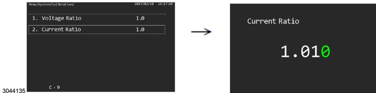
FIGURE 4-4. CURRENT RATIO CALIBRATION
