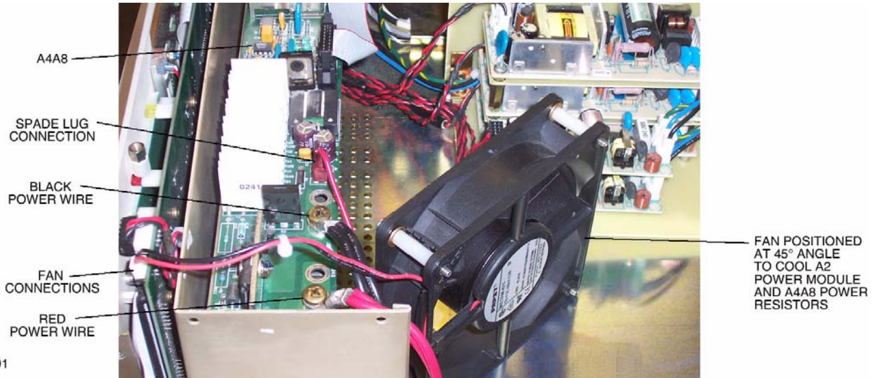
FIGURE 2. POWER AND FAN CONNECTIONS
