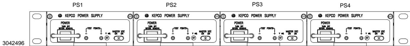
**FIGURE 2. HSF-1UR 50 WATT POWER SUPPLIES (4) INSTALLED IN RA 19-1U RACK ADAPTER**
