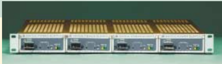
Four HSF modules shown in RA 19-1U Housing
